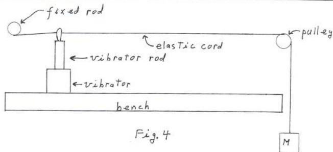
placed on the table such that the cord either passed through it, or close enough to it for the wave-driver to induce oscillations of the cord. Special care was taken to ensure that the cord did not bend due to the mechanical wave driver.
